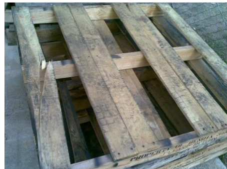
X Cracked planks
