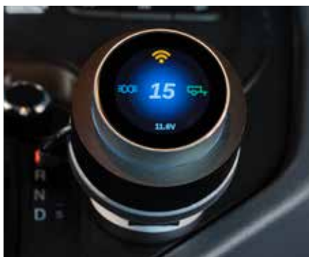
Normal Function Lights, trailer & voltage
