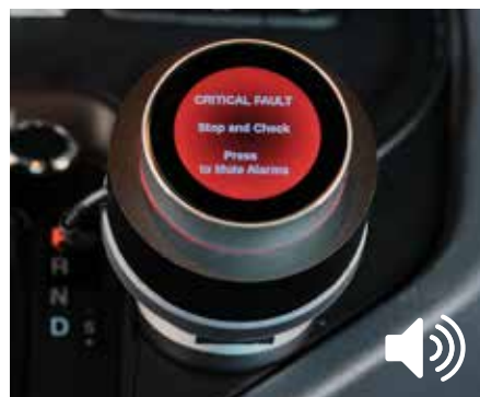
Critical Fault Check trailer wiring or lights
