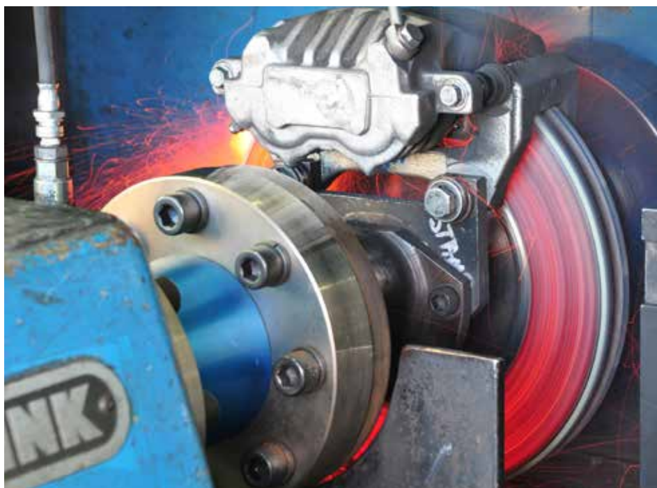
A set of Bendix brake pads is put through its paces using the company's brake dynamometer.
