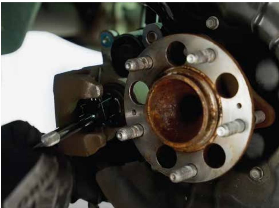
One concern for the brake system is damage to the hub flange which can lead to flange run-out, eventually causing Disc Thickness Variation.
