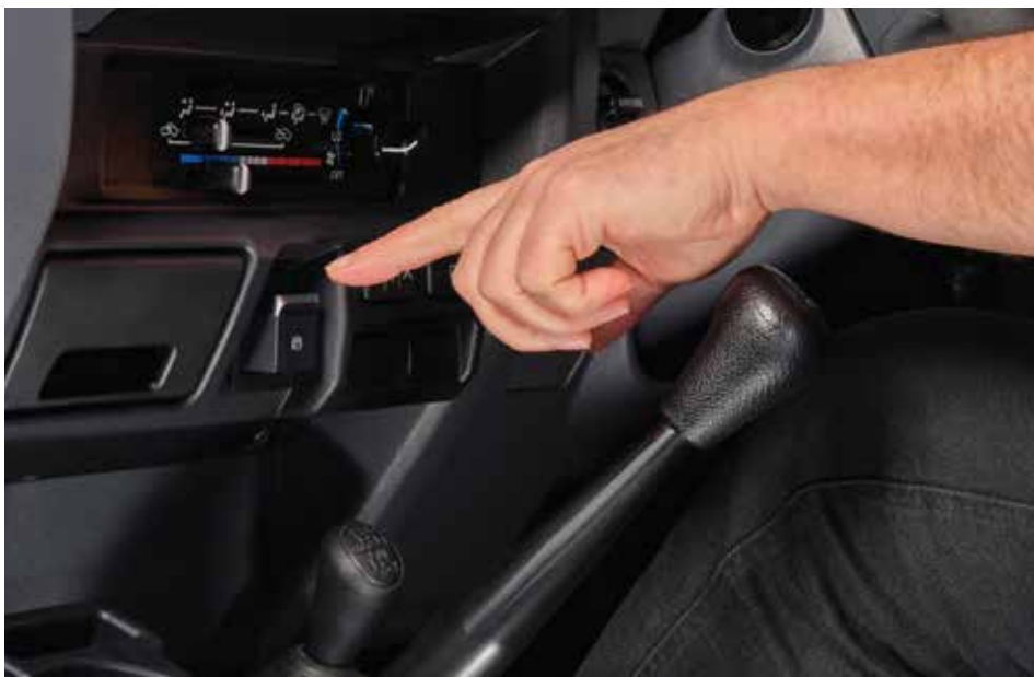
Offering complete 'bolt-on' fitment that complements the existing OE park brake, the vehicle maintains ADR-compliance. Actuating the EPB is easy using the neat, OE-look dashboard control switch.
