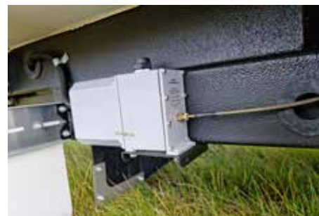
The actuator features an electric motor that drives a pump that pressurises brake fluid in the trailer's brake lines, forcing the caliper pistons and brake pads against the rotors.
