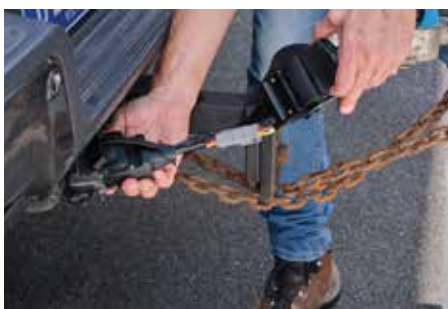
The included patch harness easily mounts between vehicles' existing seven and/or 12-pin trailer / caravan plugs, so tow vehicles don't need a hard-wired harness.
