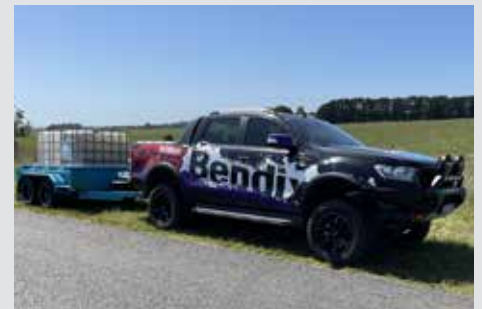
Among the on-road testing undertaken at the proving ground is a load test, where engineers assess the braking performance of the trial vehicle when coupled to a trailer loaded with up to 2,000kg of mass.
